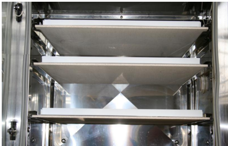
Picture 1: Test specimens in Contherm Environmental Chamber
